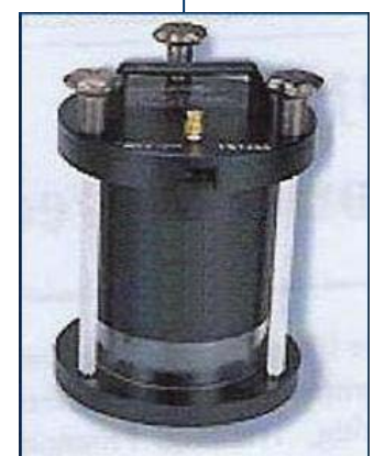
Pressure Chamber Tank
